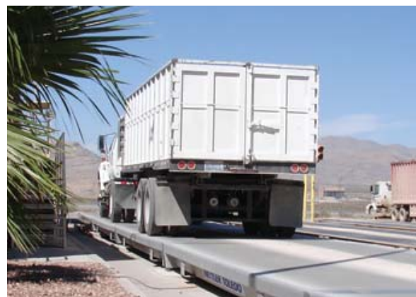
The scales at the Apex Landfill handle inbound and outbound weighing for as many as 1,200 trucks per day.
