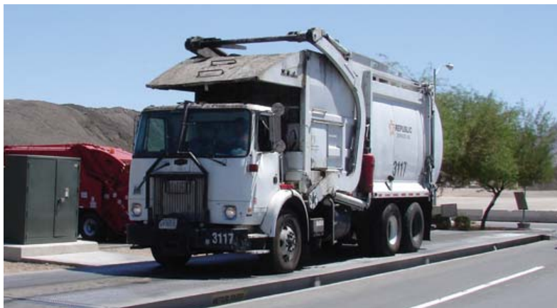
The Henderson Transfer Station uses model 7562 truck scales for inbound weighing.
