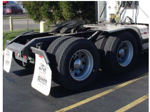
The module masher simulates how a load is applied by a truck's dual tandem axle.
